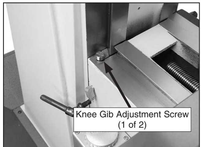
Figure 62. Knee gib adjustment screw (1 of 2).
